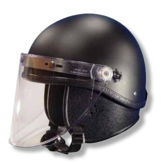
**SHELL:** FIBERGLASS partial coverage shell with multiple layer impact absorbing materials. Ear and Neck Protector permanently attached to shell. Snap attachments for Riot Control Faceshield. Three shell sizes, small/medium, large & extra large. Dull matte finish.
